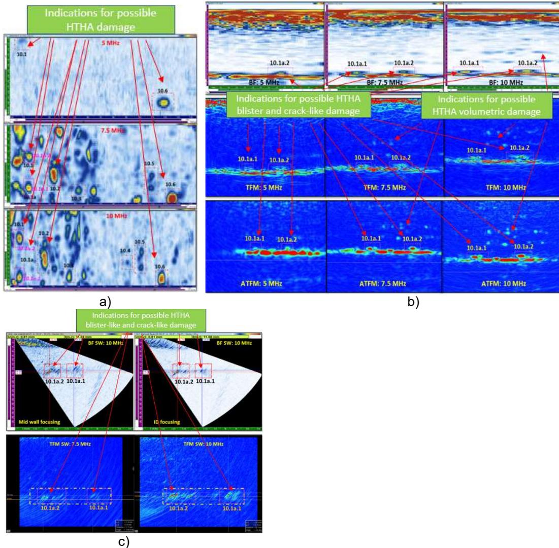
**Figure A6. Imaging of Indication #10.1a.1 and #10.1a.2: (a) projected PAUT straight beam C-Scans comparison; (b) PAUT straight beam and FMC/TFM/ATFM LL B-Scans comparison; (c) comparison of PAUT S-Scans and FMC/TFM TT B-scans using shear wave techniques.** From Materials Evaluation, Vol. 78, No.11. Copyright © 2020 by The American Society for Nondestructive Testing Inc. Reprinted with permission.
