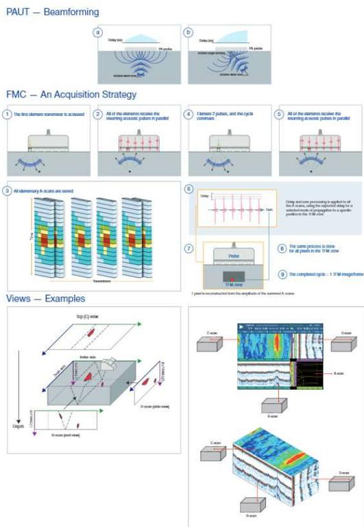
Figure A1. PAUT and FMC/TFM principals and views. Reprinted with permission from Olympus.
