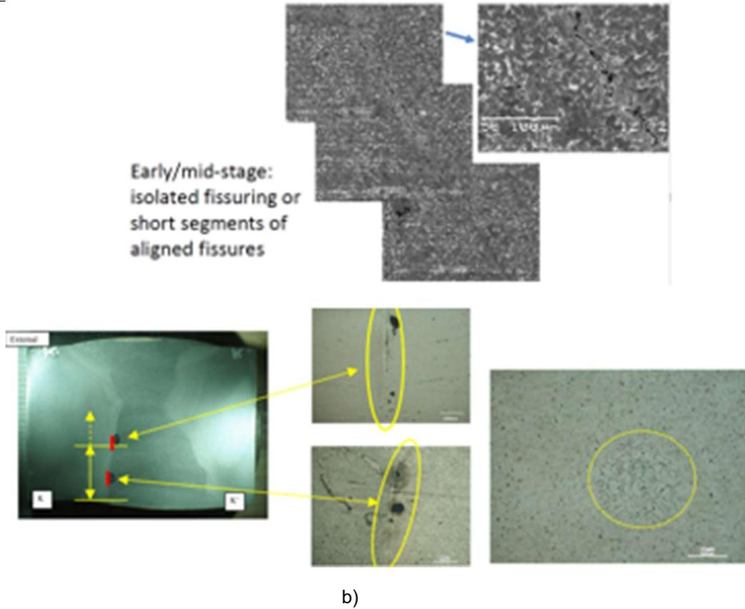
Figure B4. HTHA Imaging using: (a) TOFD - left and FMC/TFM - right; (b) optical metallography. Reprinted with permission from Sonomatic.
