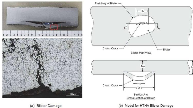
**Figure 2—HTHA Blister Damage Manifestation (left) and Sketch (right)**
