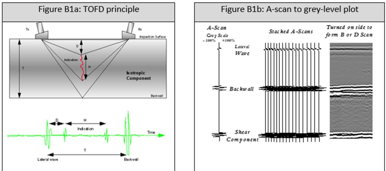
Figure B1. TOFD Principle and Presentation of Results. Reprinted with permission from Sonomatic.
