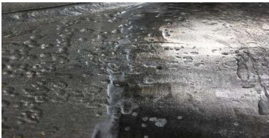
**Figure B2. Surface before grinding (left) and after grinding before grit finish (right).**
