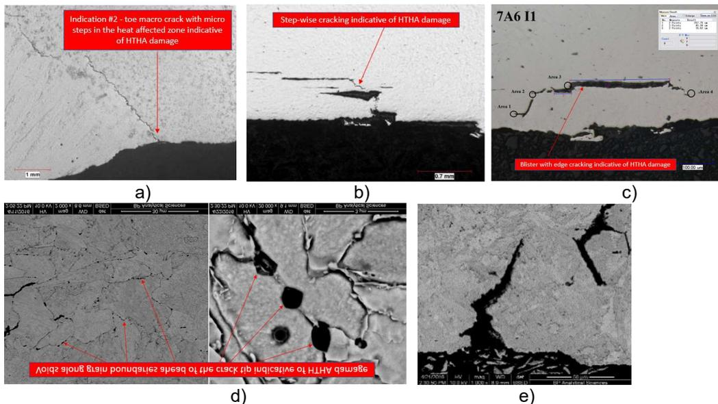
**Figure A5. Weld damage validation using optical metallography and SEM: (a) root cracking (~20X, Nital etched); (b) stepwise macro cracking (~40X, Nital etched); (c) blisters (~40X, Nital etched); (d) voids along grain boundaries (~2,000X, Nital etched-left; ~20,000X, Nital etched-right); (e) stress-related micro cracking (~1,000X, Nital etched. From Materials Evaluation, Vol. 78, No.11. Copyright © 2020 by The American Society for Nondestructive Testing Inc. Reprinted with permission.**
