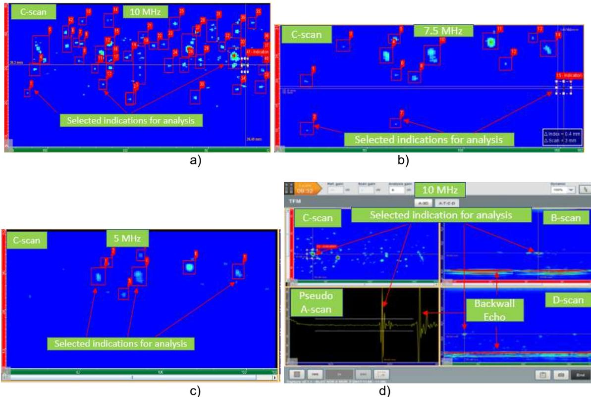
**Figure A2. FMC/TFM LL imaging: (a) 10MHz projected C-scan of damage block; (b) 7.5MHz projected C-scan of damage block; (c) (5MHz projected C-scan of damage block; d) 10MHz split screen imaging of selected indication: projected C-scan (left top), single plane B-scan (top right), single plane D-scan (bottom right), pseudo A-scan (bottom left).** From Materials Evaluation, Vol. 78, No.11. Copyright © 2020 by The American Society for Nondestructive Testing Inc. Reprinted with permission.
