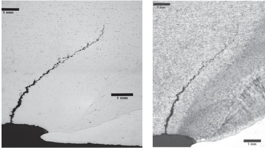
**Figure 3—HTHA Crack-like Flaw Damage Manifestation**
