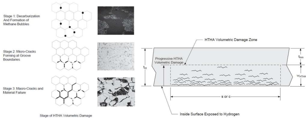
**Figure 1—HTHA Volumetric Damage Manifestation (left) and Sketch (right)**
